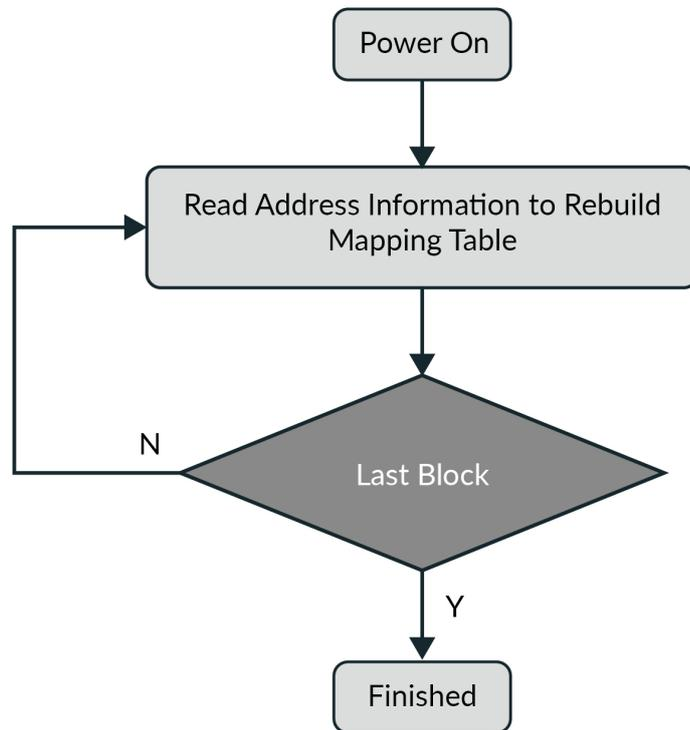
Figure 4: Mapping Table Rebuild Flow after Power On
