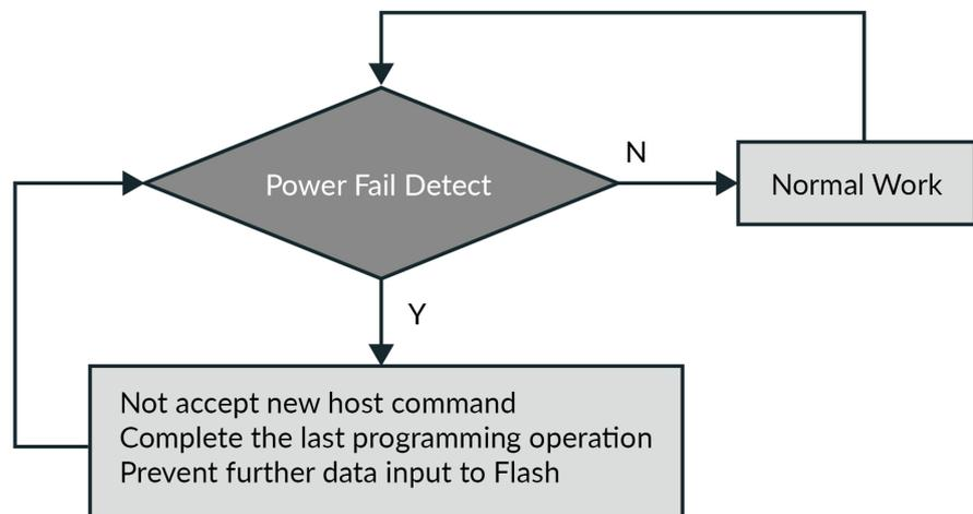
Figure 1: Power Failure Data Protection Block Diagram of Innodisk SSDs
