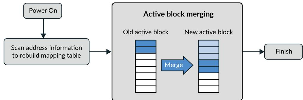
Figure 2: Power-down Recovery Algorithm Block Diagram of Innodisk SSDs
