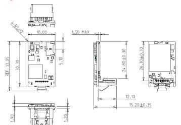
TOLERANCE: ±0.20mm UNIT: mm
